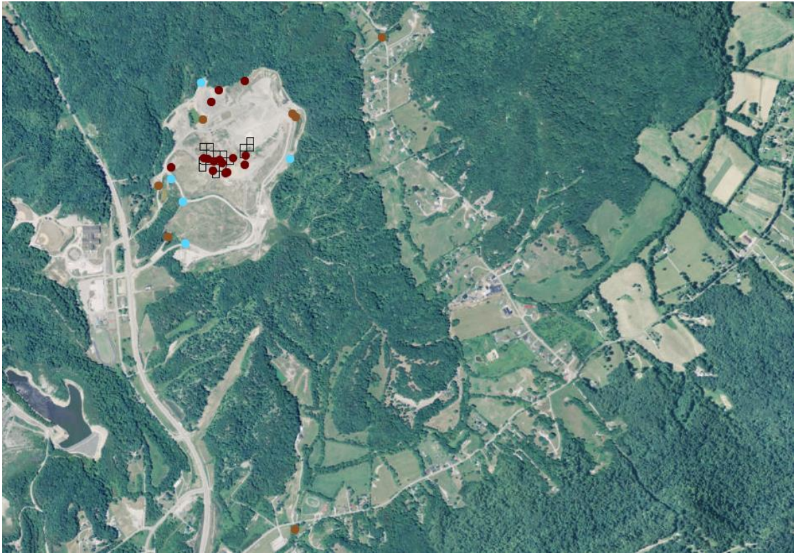
Figure 7. Soil (dark brown), sediment (light brown), and groundwater (blue) sampling locations. The waste in question was deposited in the area covered by the square grid cells.
