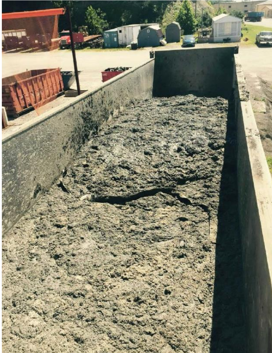
Figure 6. Sawdust solidified waste from Fairmont Brine Processing in semi-tractor trailer ready for hauling to ADS Blue Ridge Landfill (taken from Pendergrass et al. 2015).
