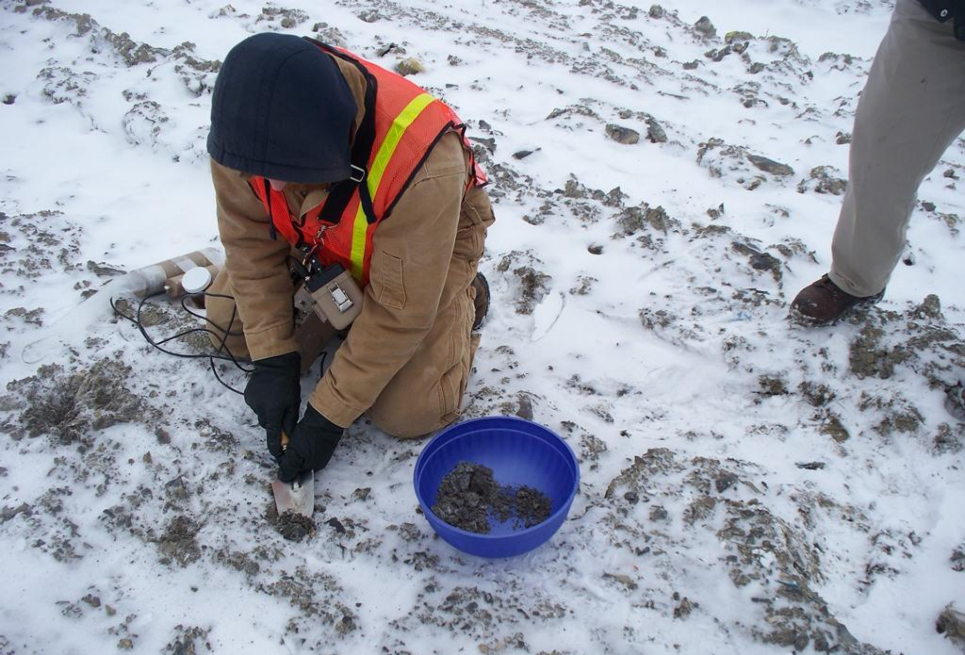
Advanced Disposal Blue Ridge Landfill AI 998 2/10/16 g. weems Taking samples to test for TENORM
