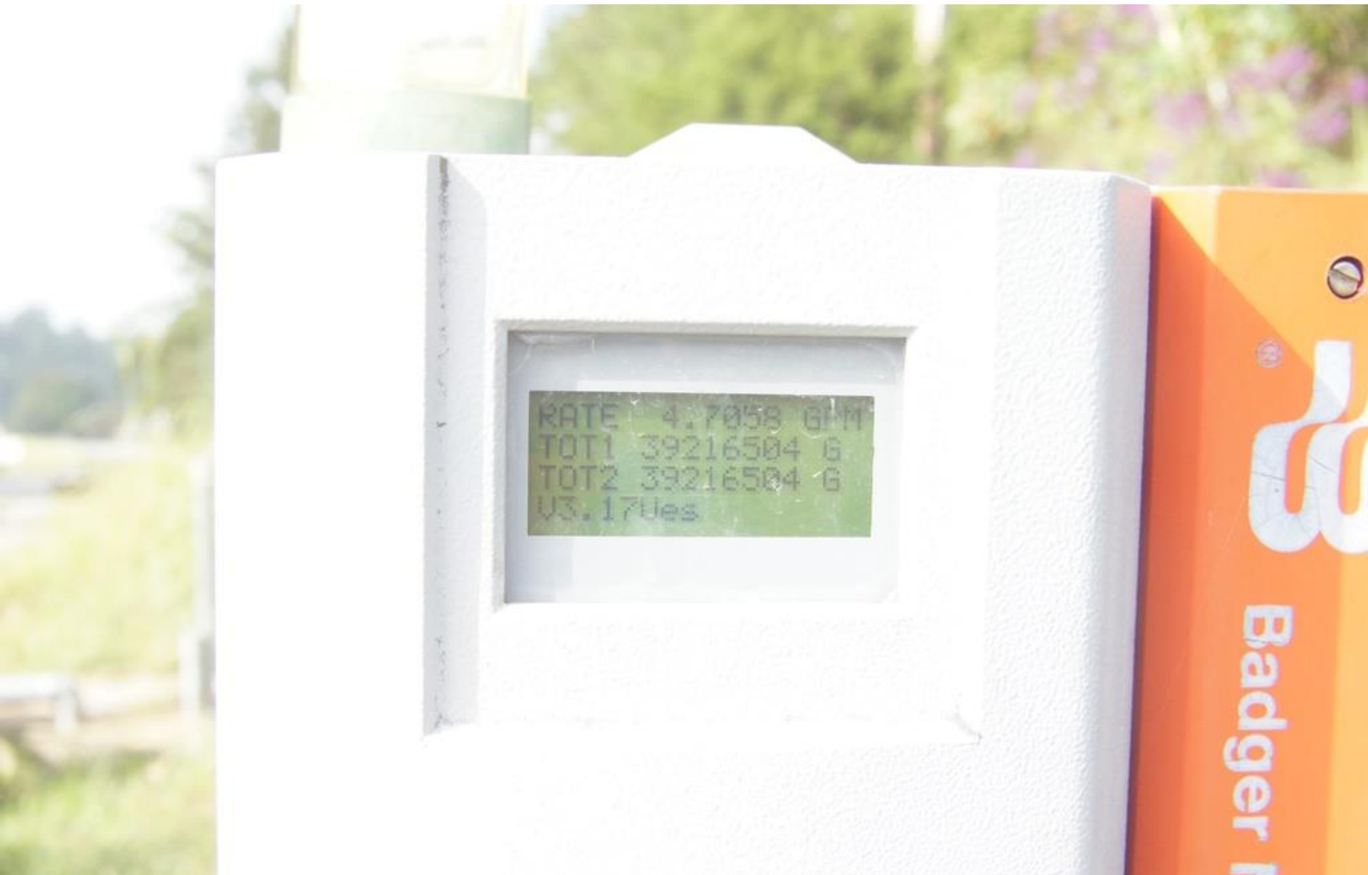
Advanced Disposal Blue Ridge Landfill AI 998 9/11/15 g. weems Flowmeter to Estill county water treatment system the Blue Ridge Landfill is connected to for disposing leachate.
